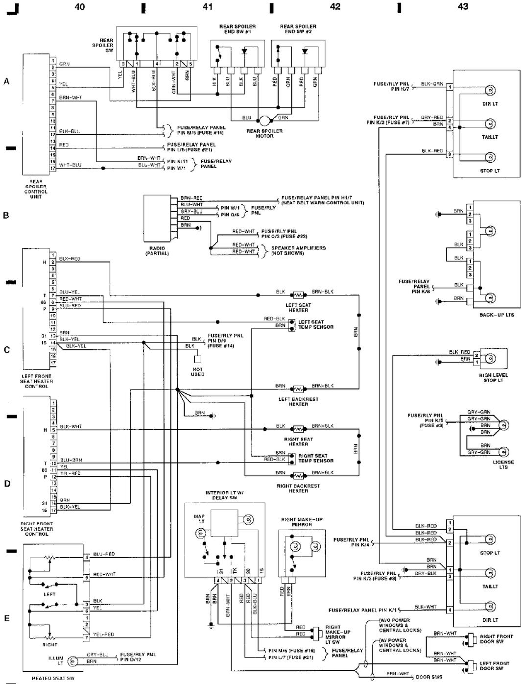
Fig. 11: Seat Heater, Spoiler Ctrl, Taillights (Grid 40-43)
